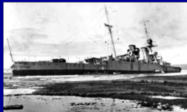
This was probably taken after the picture directly above, albeit not very long after, judging from the intact state of the ensign. Note the stream anchor still housed at the stern, which the captain had ordered out in vain.
